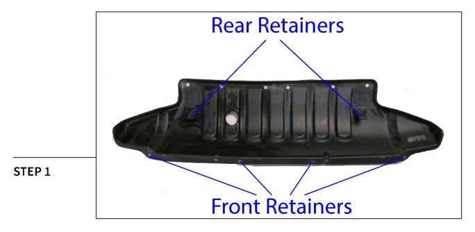
Remove the (4) front and (2) rear plastic push pin splash shield retainers. Remove splash shield from the vehicle.
