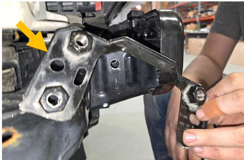
**F. Install the Maximus-3 brackets** as shown below using M12 bolt, serrated nuts and washers supplied.
