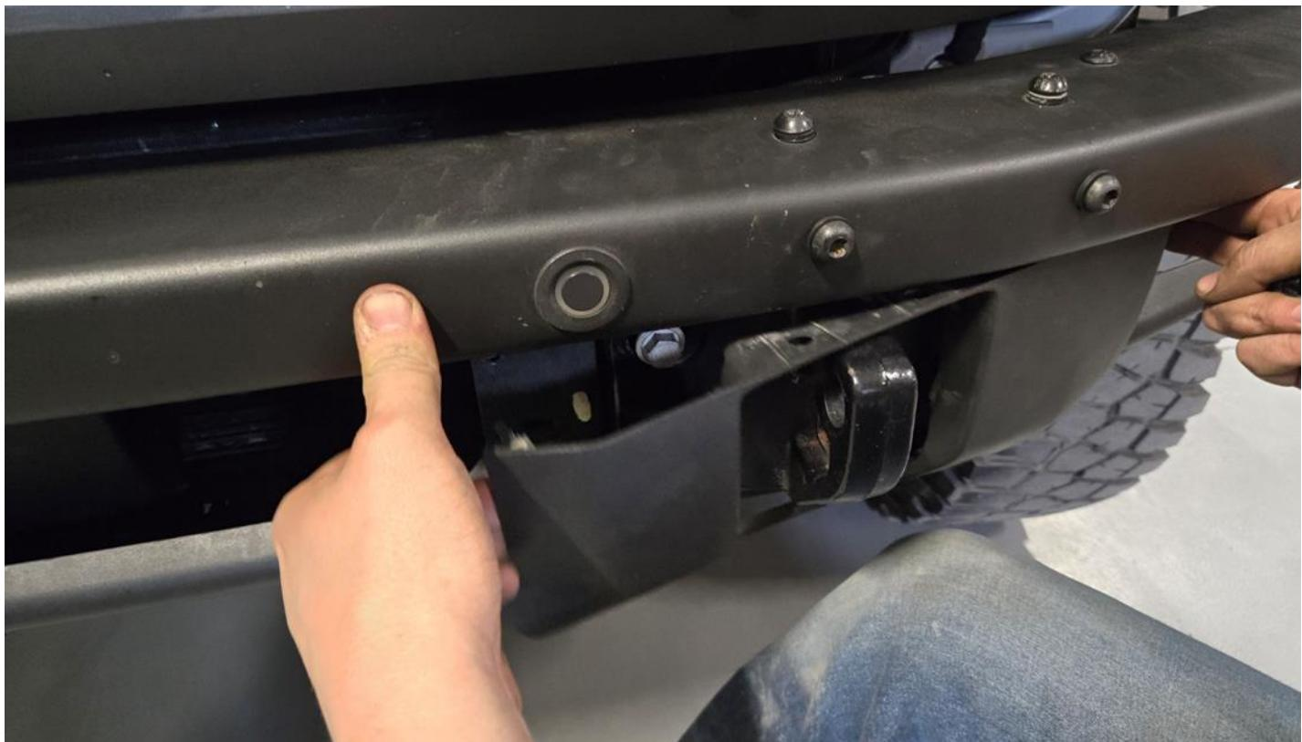
**B. For the driver side:** assemble the Slider Tab, 2 Pucks and Back Plate as shown below using M12 bolts and nuts provided. Make sure you do this with the plastic cover in place as you cannot add it later. Please note the order and orientation of the components.
