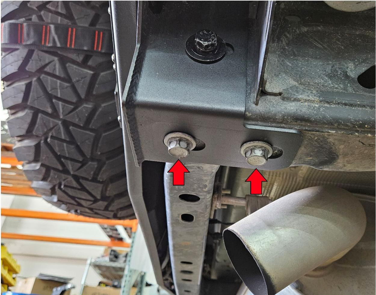
**Step 2:** Align the tow loop and spacer plate with mounting holes and start the screws. Note the position of the spacer plate between tow loop and bumper.
