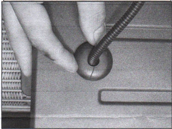
(Fig 7) Push Rubber Grommet on Harness into sensor hole (Bumper used for Example)
