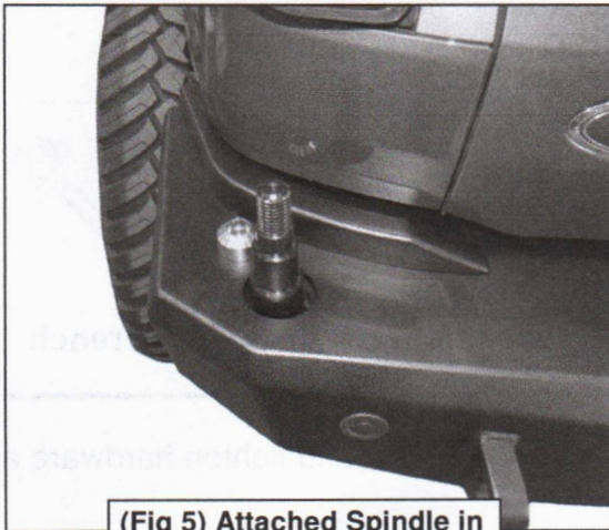
(Fig 5) Attached Spindle in Swing Arm mounting hole
