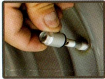
Metal Valve Stem Install
