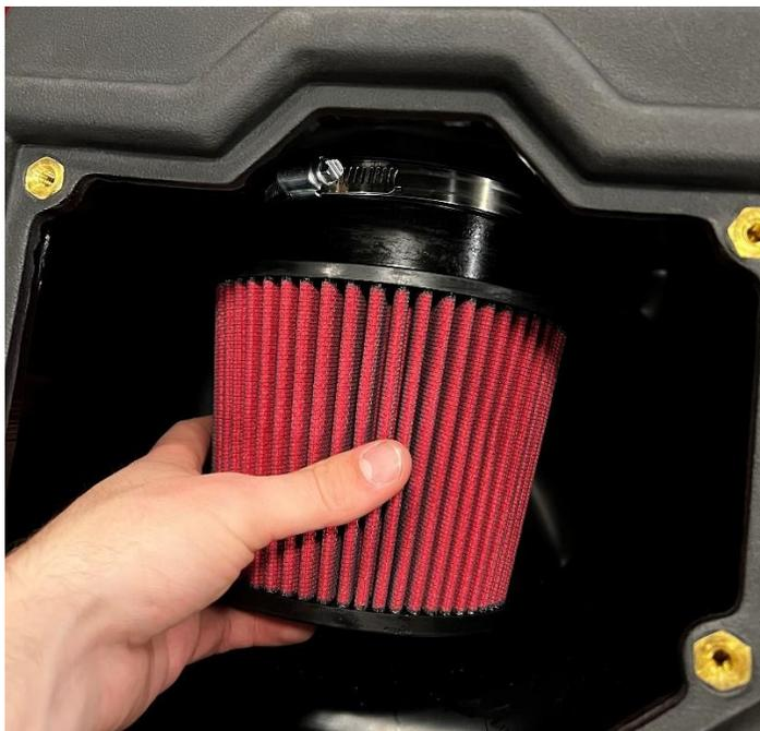
**7.** Install the air filter and air filter clamp directly over the end of the air duct inside the air box. Use an 8mm Socket to tighten. Fit pre-filter over top of filter if desired.
