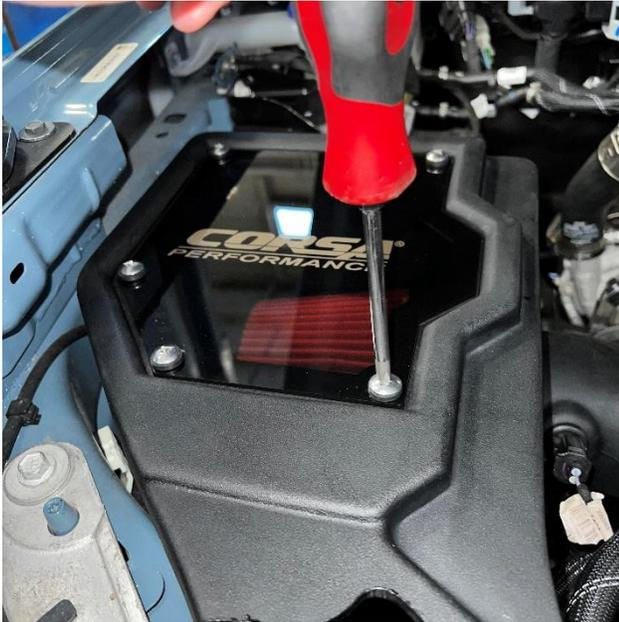
13. Place the CORSA lid on top of the airbox and tighten to the air box using the lid screws and a Phillips screwdriver.
