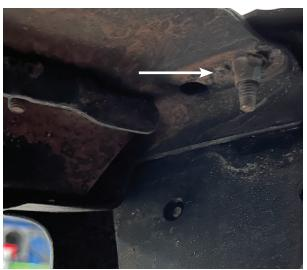
**Step 3:** Install the bracket with the lights attached into the fog light pocket. Once the bracket is lined up with the mounting locations, install the 13mm bolt. Next, using the supplied spacer and 13mm flag nut, place the bracket over the bolt in the picture, followed by the spacer and then the flange nut. Remember that the spacer will need to sit with the larger opening touching the bracket and the smaller opening touching the flange nut.
