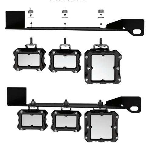
**Step 2:** Before installing the bracket with the lights, remove the 13 mm bolt from the backside of the bumper. Once the 13mm bolt has been removed, locate the other mounting point. It is located on the outer side of the fog light pocket. There won't be any hardware to remove in this location. The bracket will sit around the bolt.
