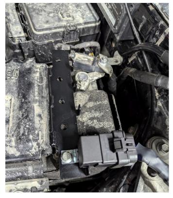
**16.** Route the pod light harnesses near the driver-side hood hinge and into the cowl. Ensure the harnesses do not get pinched when the hood is closed.
