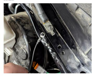
**12.** Locate the female Deutsch connector on the upfitter harness and plug it into the male connector.
