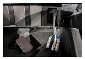
**20.** Connect the spade terminals to the switch using the included diagram. Then, press the switch into the hole until it locks in.
