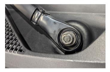
5. Remove the antenna and the four M6 cowl cover bolts.
