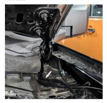
**11.** Route one of the pod light harnesses along the windshield's base over to the cowl's passenger side. Plug in the passenger side pod light. Route the other pod light harness to the driver's side of the cowl. Plug in the driver's side pod light. Tuck any excess wiring into the pocket on the driver's side of the cowl.
