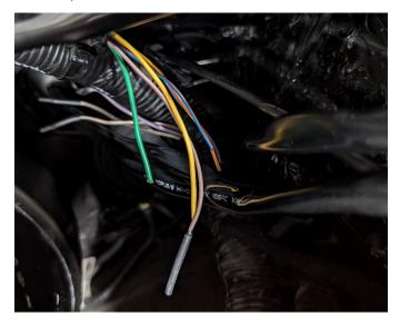
**9.** Strip off approximately one-quarter inch of insulation. Insert the wire into the female closed barrel terminal included in the kit. Ensure all the wire strands are inserted into the terminal before crimping.
