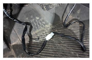
**19.** Find a suitable location for the light switch. Route the switch harness to the switch location. Pass the spade terminals out of the hole for the switch. (Optional switch panel shown)
