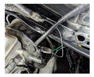
**13.** Route the upfitter harness near the driver-side hood hinge and into the cowl. Ensure the harness does not get pinched when the hood is closed.
