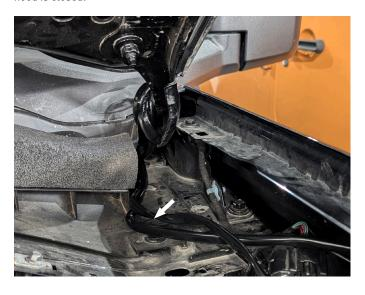
17. Route one of the pod light harnesses along the windshield's base over to the cowl's passenger side. Plug in the passenger side pod light. Route the other pod light harness to the driver's side of the cowl. Plug in the driver's side pod light. Tuck any excess wiring into the pocket on the driver's side of the cowl.
