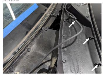
**8.** Locate the factory wiring harness on the driver's side firewall. Trim the heat shrink off the end of the green wire with the brown stripe.
