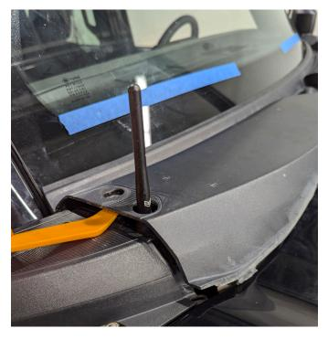
**7.** Flip the cowl cover over, disengage the windshield washer fluid hose from the two clips, and disconnect the hose. Remove the cowl cover.
