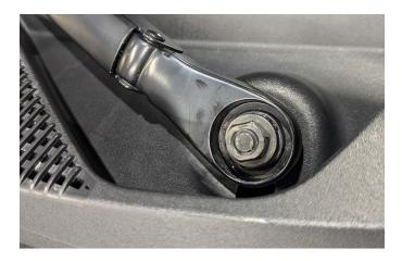
5. Remove the antenna and the four M6 cowl cover bolts.
