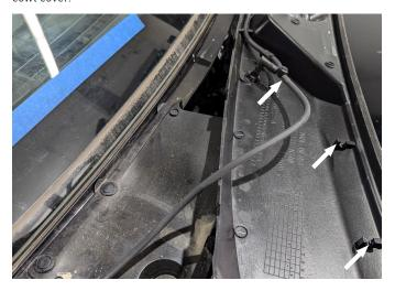
**8.** Unravel the wiring harness and locate the switch connector. Disconnect the switch harness from the wiring harness and place it off to the side for a later step.
