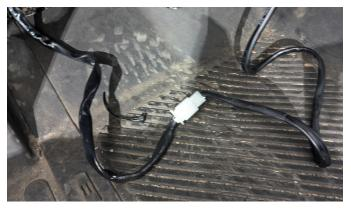
**25.** Find a suitable location for the light switch. Route the switch harness to the switch location. Pass the spade terminals out of the hole for the switch. (Optional switch panel shown)
