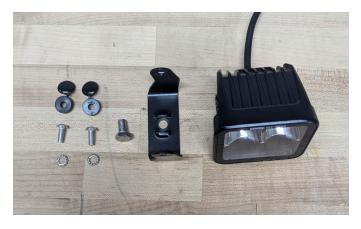
2. Insert the M8 hex bolt into the light bracket before you bolt the bracket to the pod light. Place the serrated washers between the pod light and the bracket.
