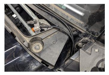
**14.** Unravel the wiring harness and locate the switch connector. Disconnect the switch harness from the wiring harness and place it off to the side for a later step.
