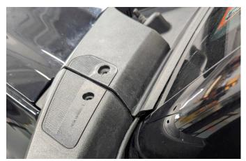
**20.** Mount the ditch light brackets using the longer M6 button-head bolts and bolt caps supplied. Tuck any excess wiring into the cowl.
