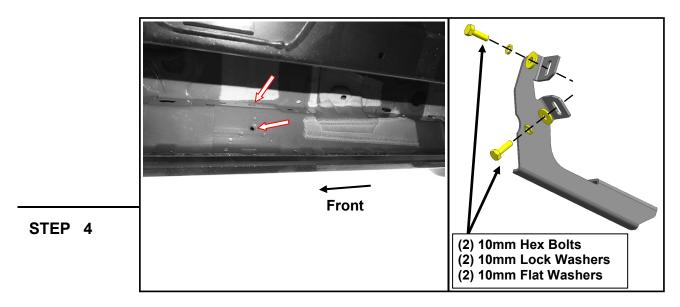
Loosely fit the (1) Passenger Rear bracket to the vehicle threaded body hole using (2) M10 x 30mm bolts, (2) M10 lock washers, and (2) M10 flat washers. Do not fully tighten to allow for later adjustments.
