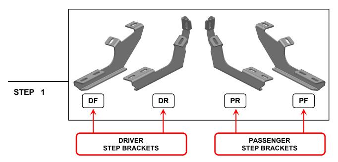
Mounting Brackets look very similar but are unique. Please identify each mounting bracket using the engraved location identifier. Note: There is a notch on the back of the Rear bracket.
