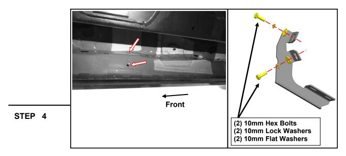
Loosely fit the (1) Passenger Center bracket to the vehicle threaded body hole using (2) M10 x 30mm bolts, (2) M10 lock washers, and (2) M10 flat washers. Do not fully tighten to allow for later adjustments. Repeat this step for the Passenger Rear bracket.
