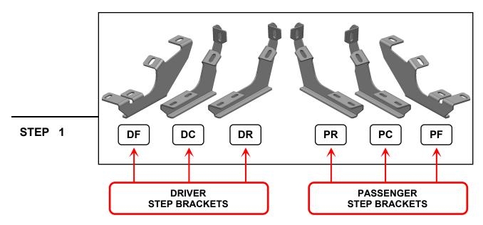
Mounting Brackets look very similar but are unique. Please identify each mounting bracket using the engraved location identifier. Note: There is a notch on the back of the Center bracket.
