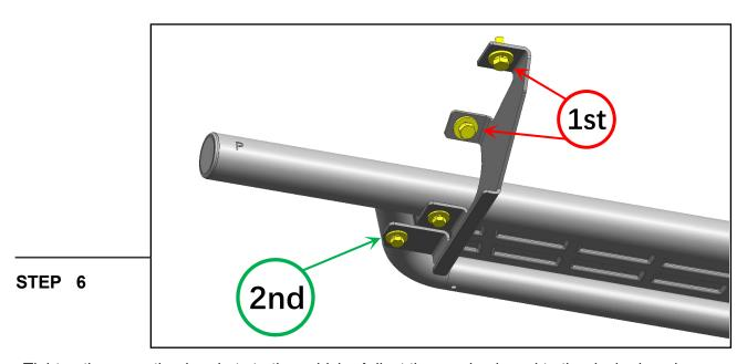
Tighten the mounting brackets to the vehicle. Adjust the running board to the desired angle, and tighten the M8 combo bolts to secure the step into place. See photo for tightening order visual.
