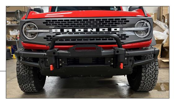
Ensure all mounting hardware is fully secure. Plug in the bumper wiring harness to the vehicle harness connector.
