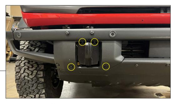
Using a panel removal tool, remove the (4) plastic push clips securing the plastic cover to the bumper.
