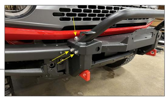
With both frame mounts loose, fit the winch plate to the frame mounts. Adjust the lower mounts as necessary. Then, secure the winch plate to each frame mount using (6) M10 x 35mm bolts, (6) M10 lock washers, and (6) M10 flat washers.
