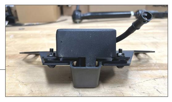
If desired, remove and relocate the vehicle forward facing camera to the included mounting bracket. Then, fit the enclosure bracket over the camera, and secure using (2) M6 x 25mm Allen bolts, (8) M6 flat washers, and (2) M6 flange nuts. Use up to (4) M6 flat washers to space the enclosure bracket away from the camera, if necessary.
