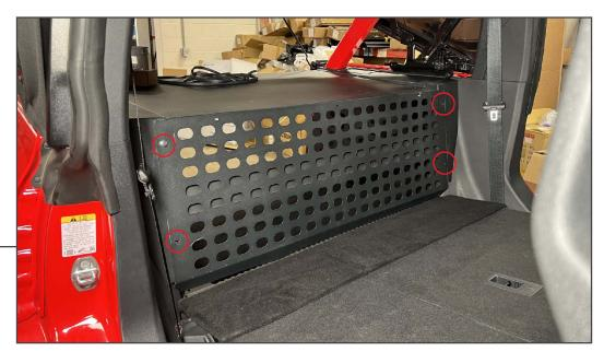
Fold the interior rear seats downwards to access the cargo area. Then, with a helper, align the center molle panel to the LH and RH 'L' brackets and secure using (2) M8 x 20mm flange bolts per side.
