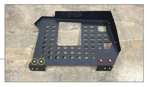
RH Side Shown Above: Assemble the bottom of the 'L' bracket to the molle panel using (2) M8  $\times$  20mm flange bolts. Assemble the RH lower mounting bracket to the molle panel using (2) M8  $\times$  20mm flange bolts.
