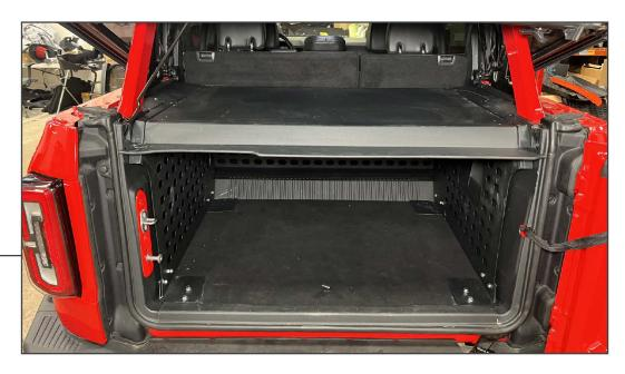
Ensure all hardware is fully tightened. Install the OEM tie down points to the top panel pre-drilled holes using (8) M8 x 20mm flange bolts and (8) M8 flange nuts.
