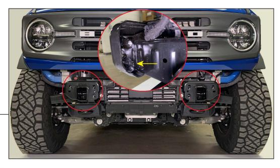
Unthread the (1) plastic wing nut from each of the bumper mounting nut plates, and remove each nut plate from the vehicle.
