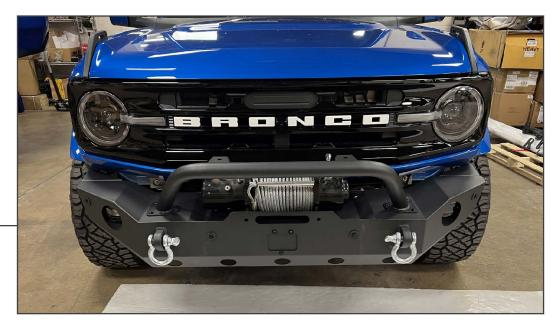
Install the (2) 3/4" D-Rings to the bumper, tighten into place. Install a winch to the bumper using the pre-drilled holes (winch sold separately).
