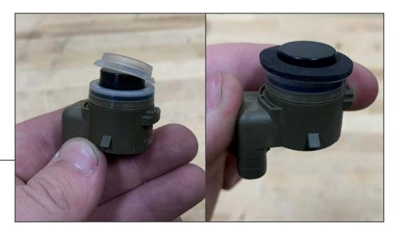
Remove the rubber gasket from around the sensor. Install the provided foam ring gasket around the sensor.
