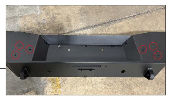
Fit and secure the over rider bar to the pre-drilled holes in the top of the bumper using (6) M8 x 25mm Allen bolts, (6) M8 lock washers, (12) M8 flat washers, and (6) M8 flange nuts. Tighten the hardware evenly until secure.
