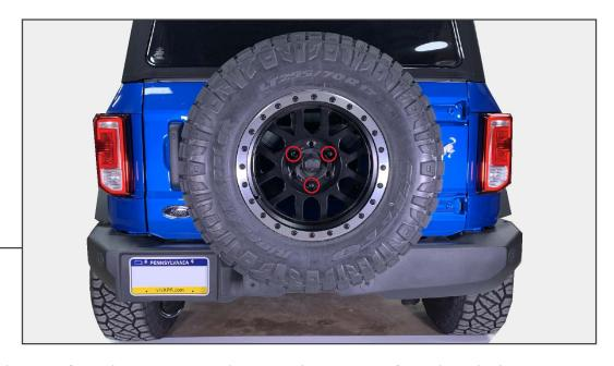
Remove the (3) lug nuts from the spare tire and remove the spare tire from the vehicle.
