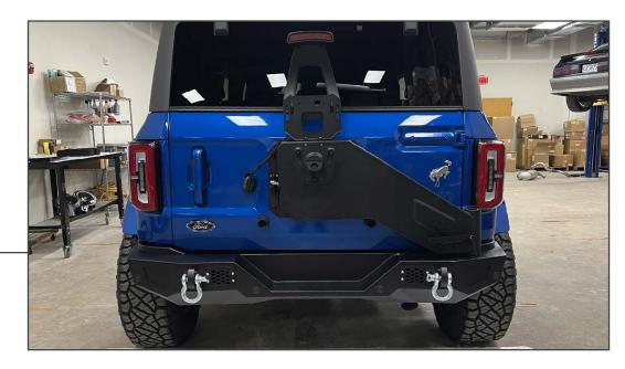
Install the (2) 3/4" D-Rings to the bumper, tighten until secure. Plug the tire carrier wiring into the vehicle harness inside the tailgate, and fit the grommet into the tailgate.
