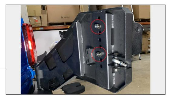
Secure the spare tire receiver bracket to the tire carrier using (2) M12 x 70mm bolts, (4) M12 flat washers, and (2) M12 lock nuts.
