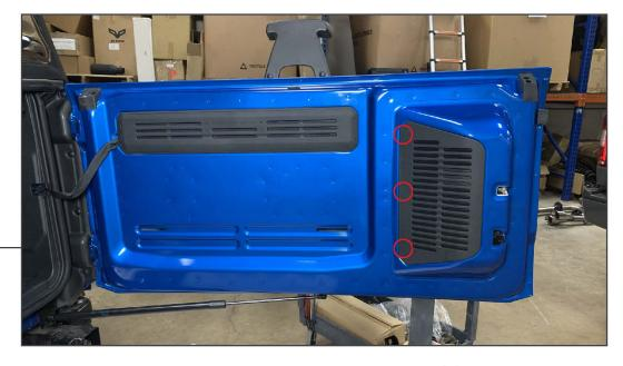
Using a plastic panel removal tool, remove the tailgate panel by dislodging (3) metal clips. Set the panel aside.
