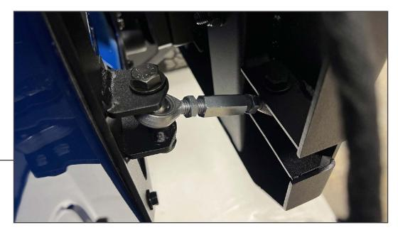
Secure the double heim joint to the tailgate mounted bracket and the tire carrier using (2) M12 x 75mm shoulder bolts, (4) M12 flat washers, and (2) M12 lock nuts. With the tailgate open, adjust the tire carrier to tailgate distance. Slowly close the tailgate until the tire carrier is tight when the tailgate is closed. Once adjusted, tighten the (2) jam nuts on the heim joint.
