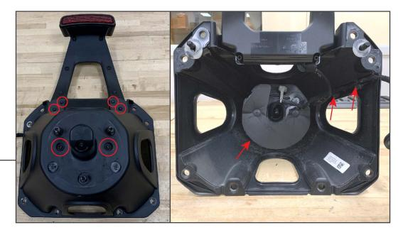
Remove (6) T-30 Torx bolts/screws from the tire carrier. Through the back of the tire carrier, dislodge the wiring harness retainers, remove the foam backing, and firmly pull the camera assembly from the tire carrier.
