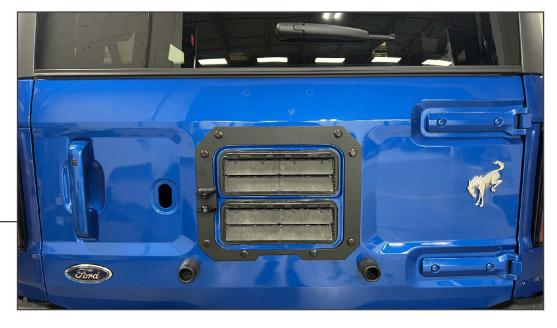
Install the included tailgate bracket to the vehicle using the original tire carrier bolts. Tighten all hardware evenly until secure.
