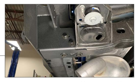
Mount the new bumper to the bottom of the vehicle frame using (4) M12 x 45mm bolts, (4) M12 lock washers, and (4) M12 flat washers. Secure the bumper to the outside of the vehicle frame using (4) M10 x 35mm bolts, (4) M10 lock washers, and (4) M10 flat washers.
