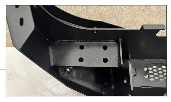
Locate the bolt holes along the RH side of the bumper. Fit the included tire carrier post, and secure into place using (4) M12 x 50mm bolts, (4) M12 lock washers, and (4) M12 flat washers. Tighten the hardware evenly until secure.
