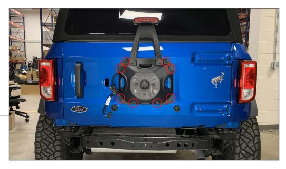
Remove (8) 13mm bolts from the tire carrier assembly. Set the tire carrier aside for disassembly later.
