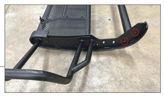
Loosely secure the center support tube to the LH and RH bumper panels using (4) M8 x 35mm bolts, (8) M8 flat washers, and (4) M8 lock nuts.
