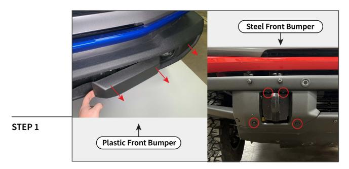
Using a panel removal tool, remove the bumper plastic trim panels covering the bumper mounting bolts.
