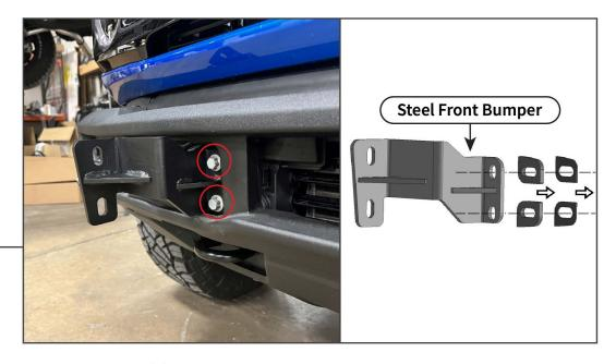
Plastic Bumper: Loosely secure the (2) lower mounting brackets to the vehicle reusing the original (2) 15mm bolts.
