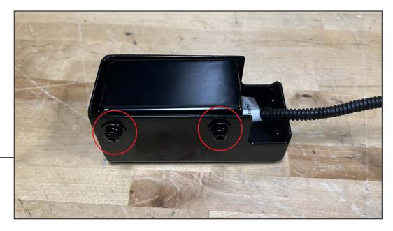
For vehicles with OEM Proximity Sensors: Secure the housing bracket to the relocation bracket using (2) M6 x 20mm combo Allen bolts.
