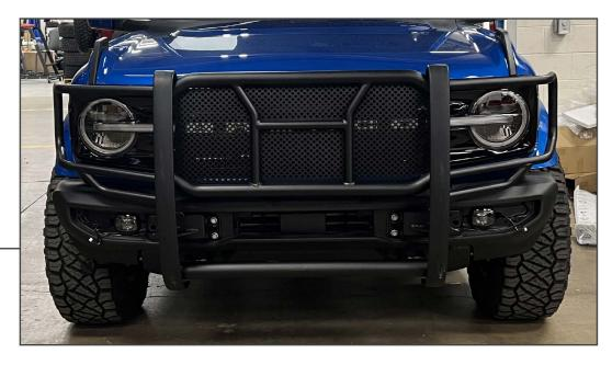
Re-install the OEM radiator cover to the vehicle reusing the original hardware. Close the vehicle hood. Adjust the grille guard to best fit the vehicle, and tighten all grille guard and mounting bracket hardware.
