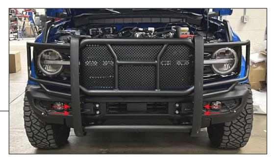
With assistance, carefully lift the grille guard assembly to the vehicle mounting brackets. Loosely secure the bottom of the grille guard to the lower mounting brackets using (4) M12 x 35mm bolts, (8) M12 flat washers, and (4) M12 lock nuts.
