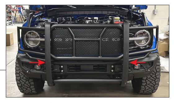
Steel/Modular Front Bumper Brackets: If equipped, secure the middle mounting brackets to the grille guard using (1) M8 x 25mm Allen bolt, (2) M8 flat washers, and (1) M8 lock nut per side.
