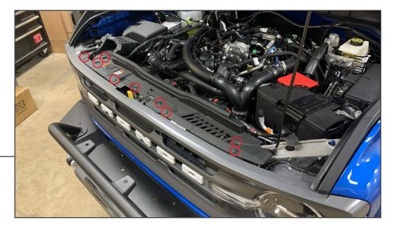
Open the vehicle hood. Remove (9) plastic push clips from the radiator cover.
