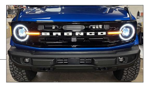
Re-install the vehicle grille and radiator cover following steps 1-3 in reverse order reusing the original hardware.
