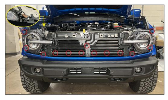
If equipped, unplug the front camera and washer line from the grille assembly.
