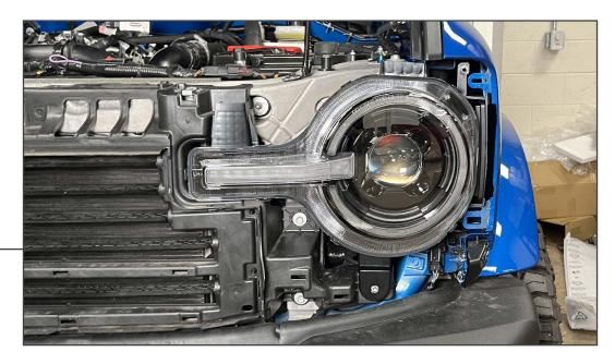
Plug the new headlight harness into the vehicle wiring harness. Then, fit the new headlight to the vehicle, ensuring the side marker harness is accessible. Secure the headlight into place using the original hardware.
