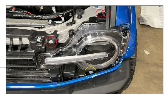
Remove (1) 10mm screw, (1) 10mm bolt, (1) 8mm screw, and (1) plastic push clip from the head-light assembly. Firmly pull the headlight assembly away from the vehicle to dislodge the retainer clip. Unplug the headlight electrical connector harness from the headlight.
