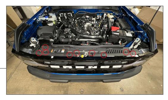
Open the vehicle hood. Remove (9) plastic push clips from the radiator cover. Then, remove the cover from the vehicle.
