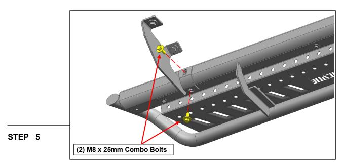
With all brackets loosely mounted to the vehicle, fit the running board onto the brackets, and loosely secure into place using (4) M8 x 25mm combo bolts.
