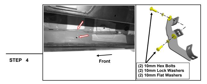
Loosely fit the (1) Passenger Rear bracket to the vehicle threaded body hole using (2) M10 x 30mm bolts, (2) M10 lock washers, and (2) M10 flat washers. Do not fully tighten to allow for later adjustments.
