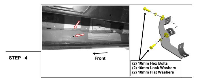
Loosely fit the (1) Passenger Center bracket to the vehicle threaded body hole using (2) M10 x 30mm bolts, (2) M10 lock washers, and (2) M10 flat washers. Do not fully tighten to allow for later adjustments. Repeat this step for the Passenger Rear bracket.
