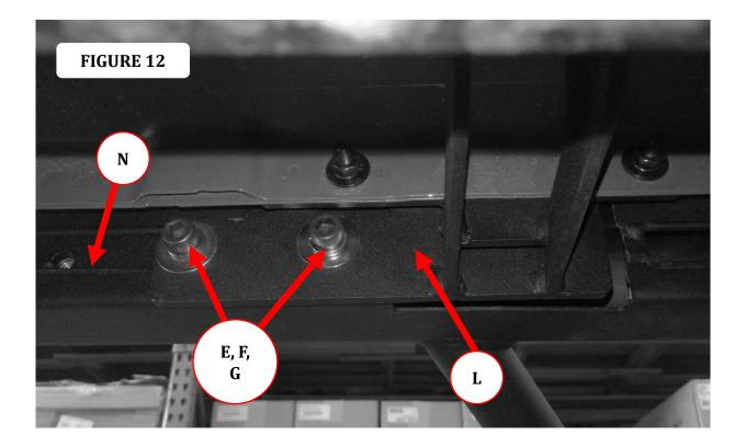
**Step-10** Align the Dominator running board with the vehicle and tighten all bolts securing the running board to the front, center and rear brackets. Repeat the above steps to install the passenger side brackets and running board. Remember to check and retighten the nuts and bolts every six months.
