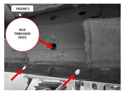
**Step-4** Attach the driver side Center bracket to the pinch mold using (2)  $1/4" \ge 1"$  hex head bolts, (4) 1/4" flat washers, (2) 1/4" lock washers and (2) 1/4" hex nuts, and to the underside of the body using (1) M10 x 25mm hex bolt, (1) M10 lock washer and (1) M10 flat washer, (FIGURE 6 & 7). Leave the nuts and bolts loose for final adjustment.
