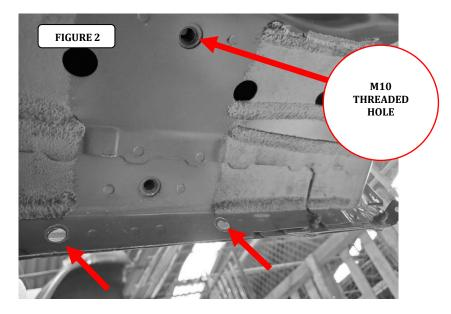
**Step-2** Attach the driver side Front bracket to the pinch mold using (2) 1/4" x 1" hex head bolts, (4) 1/4" flat washers, (2) 1/4" lock washers and (2) 1/4" hex nuts, and to the underside of the body using (1) M10 x 25mm hex bolt, (1) M10 lock washer and (1) M10 flat washer, (FIGURE 3 & 4). Leave the nuts and bolts loose for final adjustment.
