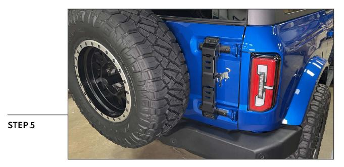
Secure the step assembly to the mounting brackets using (4) M8 x 25mm Allen bolts, (4) M8 lock washer, and (4) M8 flat washers.
