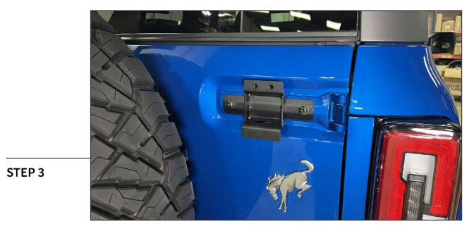
Secure the upper mounting bracket to vehicle tailgate hinge using (2) M8 x 45mm Allen bolts. Tighten the bolts evenly until secure.
