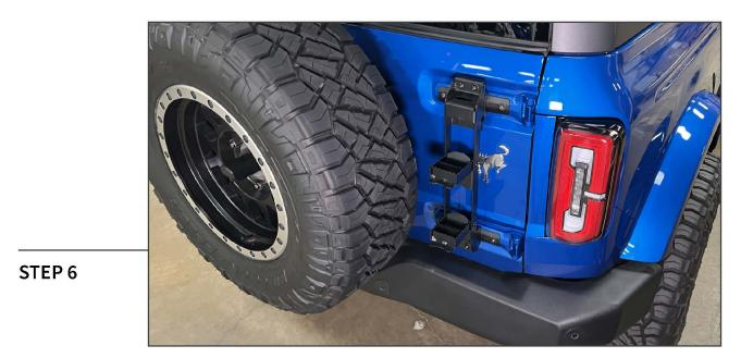
Ensure all hardware is secure. Fold the step pegs down to utilize the steps. Fold the step pegs upwards when not in use.
