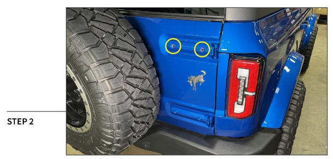
Remove (2) T-45 Torx bolts from the upper mounting bracket.
