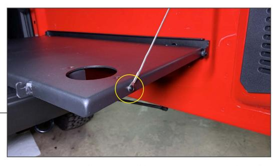
Secure the hanging straps to the bottom of the tray using (1) M5 x 14mm Allen bolt and (2) M5 flat washers, and (1) M5 lock nut per strap.
