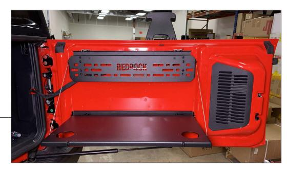
Use the upper latches to secure the table when not in use.
