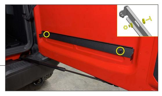
Mount the lower mounting plate to the vehicle tailgate using (2) M6 x 20mm 'T' studs w/ plastic retainers, (2) M6 spacers, (2) M6x18x1.6mm flat washers, (2) M6 lock washers, and (2) M6 hex nuts. Fit the stud base behind the tailgate slots, then tighten each M6 nut until the mounting plate is secure. Ensure the stud base is turned 90 degrees from the slot for full engagement.
