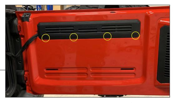
Open the vehicle tailgate. Clean the tailgate using exterior detailer and a microfiber cloth. Once clean and dry, dislodge the (4) clips to remove the upper plastic panel from the vehicle.
