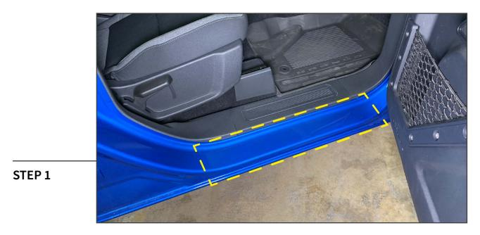
Using the designated door sill cover, test fit the cover to the vehicle before removing the adhesive tape.
