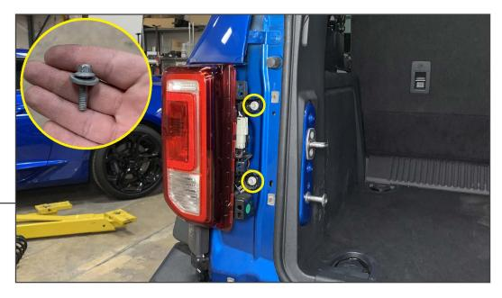
Remove (2) 8mm bolts from the inside of the tail light assembly. Firmly pull the tail light assembly away from the vehicle body to dislodge the alignment pins.
