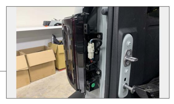
Carefully fit the tail light into the vehicle mounting position, ensuring all alignment points are fully engaged. Then, secure the tail light to the vehicle using the (2) original 8mm bolts. Tighten the hardware evenly until secure.
