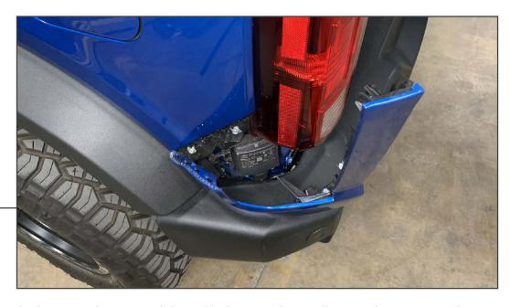
Pull outwards on the horizontal portion of the tail light trim, then pull upwards to remove the trim from the vehicle.
