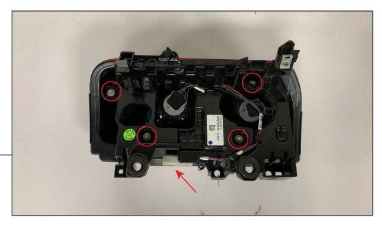
Lift the retaining tab, and slide the wiring harness connector from the post. Then, un-route the wiring harness from the tail light bracket.
