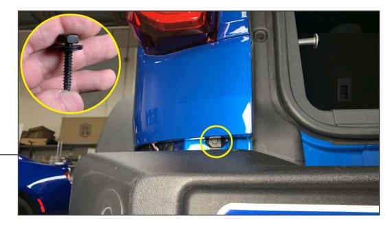
In between the vehicle body and the rear bumper, remove (1) 10mm bolt.
