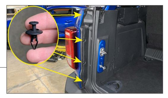
Remove (4) Phillips head plastic push clips. Loosen the Phillips head inner portion of the clip, then pull the plastic clip body out of the vehicle.
