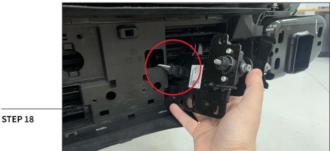
Unplug the ACC module from the shutter assembly wiring harness.
