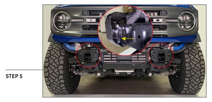
Unthread the (1) plastic wing nut from each of the bumper mounting nut plates, and remove each nut plate from the vehicle.
