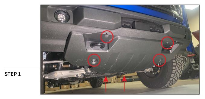
Remove (6) 15mm bolts from the lower splash shield.
