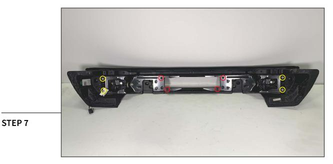
Remove (4) 10mm bolts and (4) 15mm bolts to remove the rear bumper brace to reveal the fog light harness from the bumper assembly.
