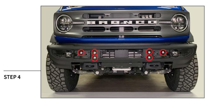
Remove (6) 15mm bolts from the front bumper, and remove the bumper assembly from the vehicle.
