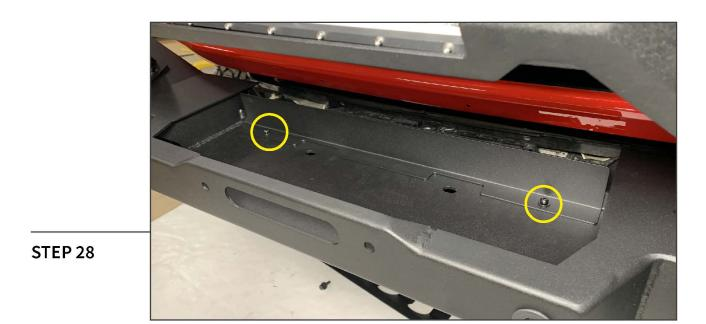
Install the shutter block-off plate to the winch area of the bumper using (2) M6 x 20mm combo Allen bolts, (2) M6 flat washers, and (2) M6 flange nuts. Tighten the hardware until secure.
