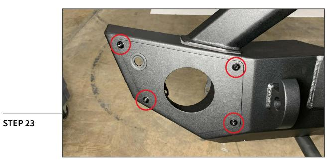
Secure each fog light mounting panel to the bumper using (4) M6 x 20mm combo Allen bolts, (4) M6 flat washers, and (4) M6 flange nuts. Tighten all hardware evenly until secure.
