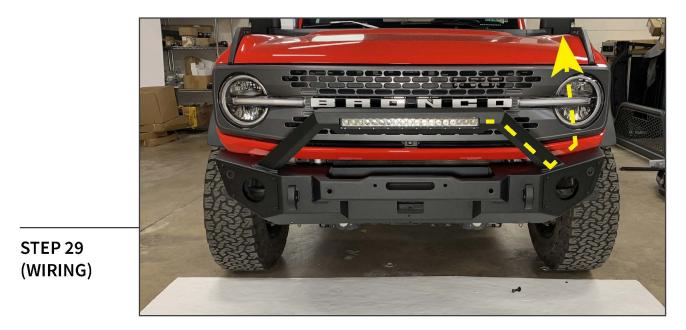
Open the vehicle hood. Route the included wiring harness from the LED light bar into the engine bay towards the vehicle battery/cabin.
