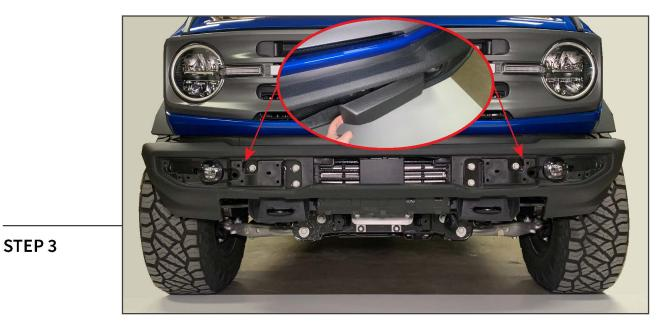
Remove the (2) plastic bumper covers using a plastic panel removal tool to reveal the bumper mounting hardware.
