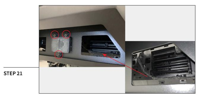
Mount the ACC module to the bumper using (3) M6 x 25mm bolts, (3) M6 flat washers, and (3) M6 flange nuts, tighten until secure.
