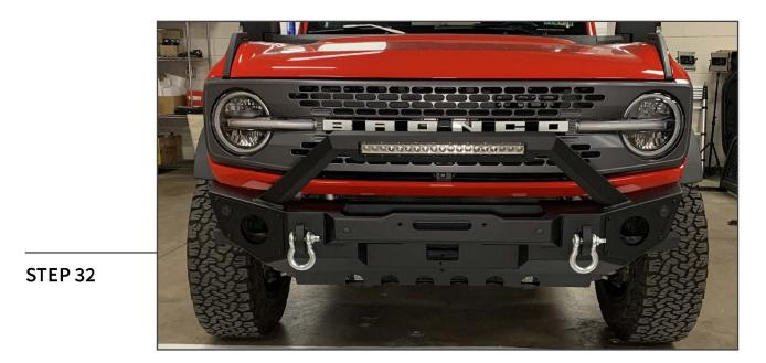
Install the (2) 3/4" D-Rings to the bumper mounting points, ensure the rings are tight using leverage.
