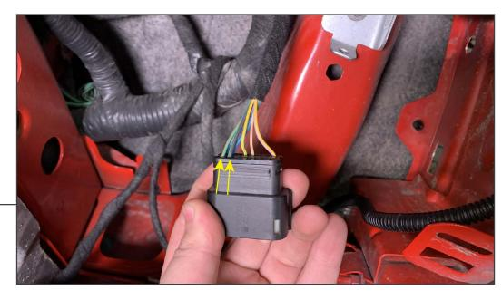
Splice the fog lights into the vehicle parking lamp circuit in the vehicle headlight connector using the (2) scotchlok connectors following the diagram below. The lights will power on with the vehicle parking lamps.
