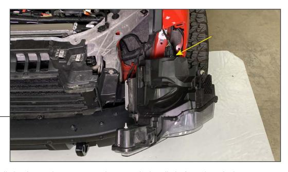
Unplug the headlight electrical connector, and remove the headlight from the vehicle.
