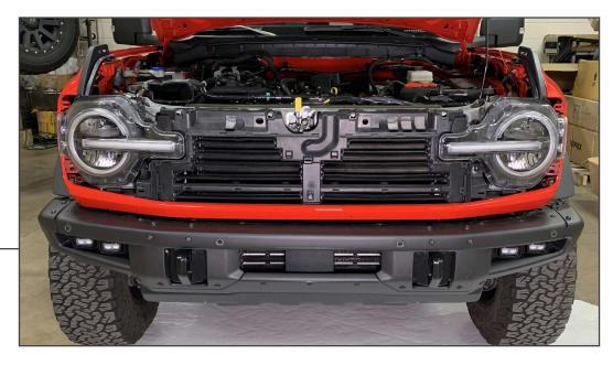
Firmly pull the grille away from the vehicle to dislodge the retaining clips. Set the grille aside on a soft surface.
