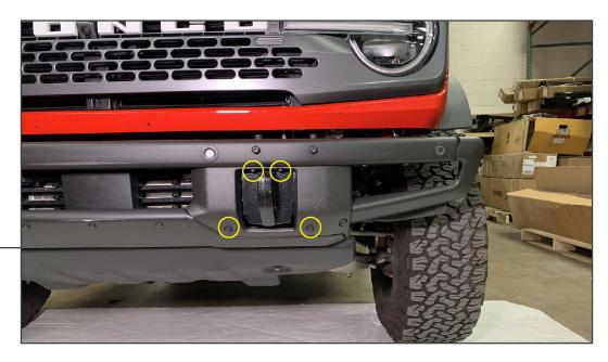
Using a panel removal tool, remove the (4) plastic push clips securing the plastic bumper cover to the bumper. With the clips removed, firmly pull the plastic panel to remove from the bumper.
