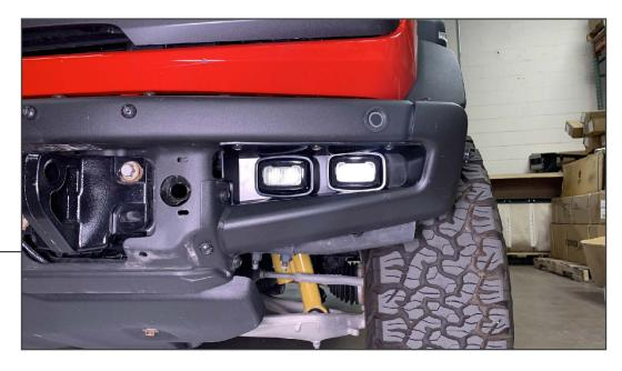
Route the fog light assembly into the back of the bumper, and secure into place using the original (3) T-40 Torx bolts. Tighten the hardware evenly until secure. Re-install the plastic cover using the bumper using OEM plastic push clips.
