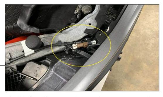
If vehicle is equipped with the forward facing camera, disconnect the camera connector and washer line fitting.
