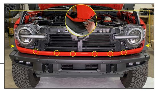
Firmly pull the side of the front painted trim panel to dislodge the panel from the vehicle fender retainer on each side. Then, pull firmly along the center of the painted trim panel to dislodge the retaining clips. Remove the painted trim panel and set aside on a soft surface.
