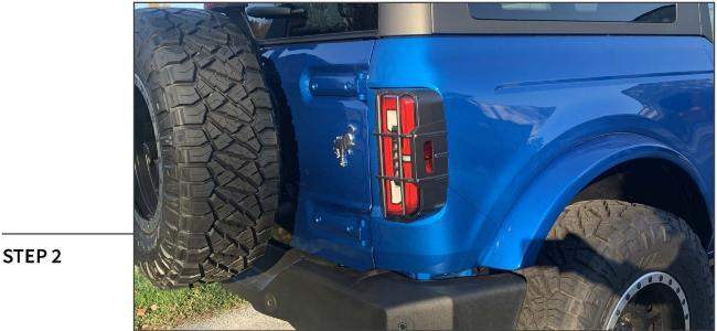
Test fit the tail light guard to the vehicle before removing the tape backing to familiarize fitment.
