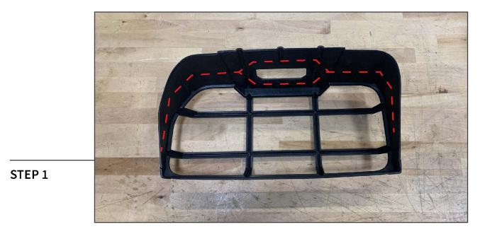
Clean the inside of the tail light guard using (1) alcohol prep pad, then (1) adhesion promoter prep pad, and allow to dry. Apply the included double sided tape to the tail light guard.
