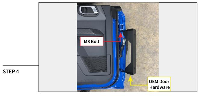
Remove the door from the vehicle following the OEM door removal procedure. Lift the door to the mounted door bracket and fit the bottom door hinge into the M6 dowel. With the door in the lower dowel, secure the top of the door using the included (1) M8 bolt.
