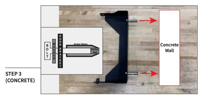
Find the appropriate mounting position along the concrete wall. Once located, align the mounting bracket to the wall, and mark the (2) holes on the wall using a pencil. Pre-drill the holes using a 15/32" drill bit. Fit the anchors to the door bracket, and into then into the drilled holes. Tighten the anchors to secure the door bracket to the wall.
