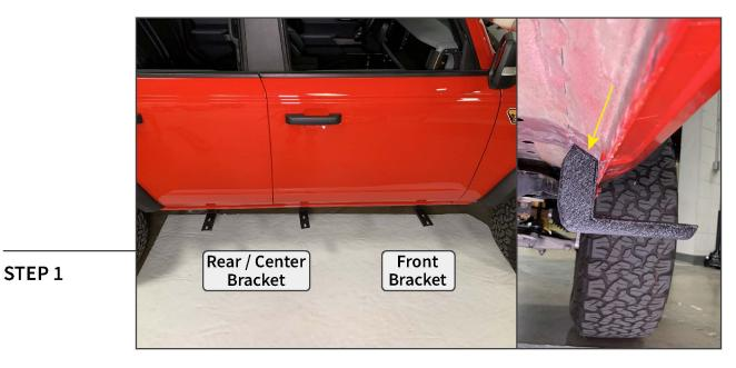
Identify the mounting brackets. The front mounting brackets are smaller than the rear/center brackets.
