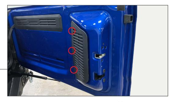
Open the vehicle tailgate. Remove the rear plastic trim by dislodging the (3) retainers. Set panel aside for re-installation later.
