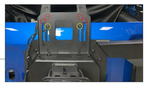
Remove the third brake light assembly from the original tire carrier by removing (4) T-30 Torx screws. Once removed, install the third brake light assembly to the new tire carrier bracket using the OEM T-30 Torx screws. Install the provided (2) #12 Phillips screws and (2) flat washers into the third brake light for additional support.
