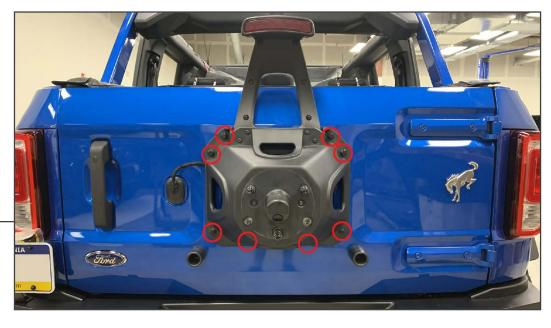
Close the vehicle tailgate. Remove (8) 13mm bolts to remove the original vehicle tire carrier from the vehicle. Set aside for disassembly later.
