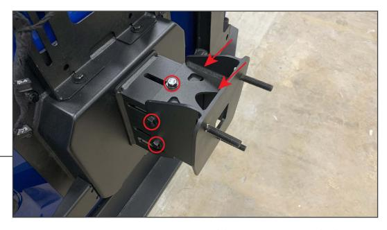
Secure the spare tire mount to the intermediate bracket using (5) M10 x 30mm bolts, (10) M10 flat washers, and (5) M10 lock nuts.
