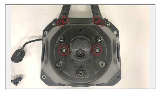
Remove (6) T-30 Torx screws to disconnect the third brake light and the backup camera from the spare tire carrier.
