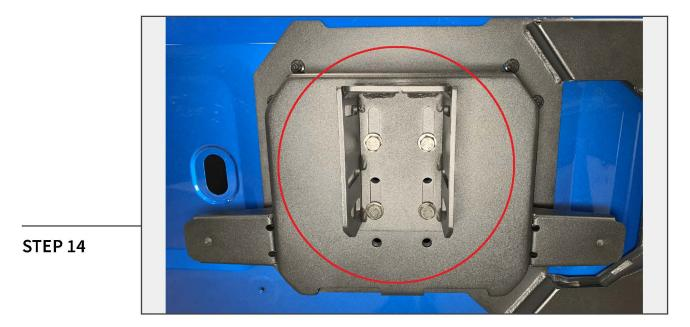
Install the (1) intermediate bracket to the tire carrier using (4) M12 x 40mm bolts, and (4) M12 flat washers.
