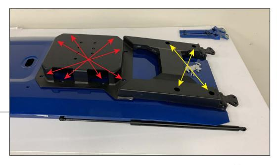
Place the tire carrier onto the vehicle tailgate. Secure the tire carrier using the original (8) 13mm bolts for the middle. Secure the RH side of the tire carrier using (4) M8x1.25 x 30mm combo bolts.
