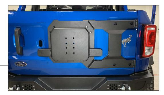
Install the vehicle tailgate to the vehicle using the (4) original hinge bolts.
