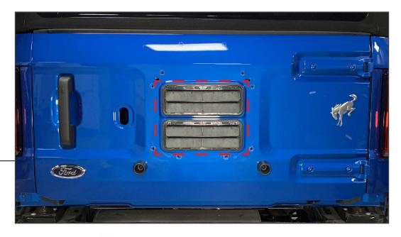
Using a plastic pry tool, remove the (2) tailgate vents.
