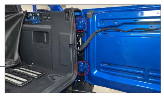
Use masking tape and a permanent marker to indicate tailgate alignment with the vehicle. Once indicated, remove the (4) tailgate mounting bolts. Lift and remove the tailgate from the vehicle and set on a soft surface.
