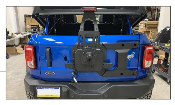
Test fit the spare tire, and adjust the tire carrier as necessary to allow proper adjustments of the spare tire depth / spare tire bumpers, and third brake light height.
