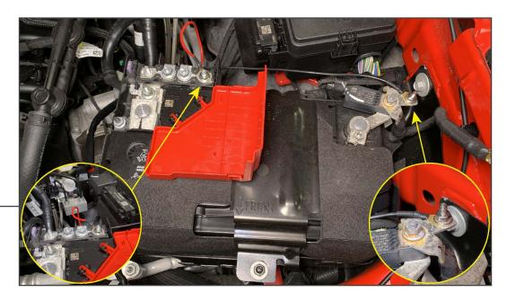
Connect the wire lead terminals to the vehicle battery.
