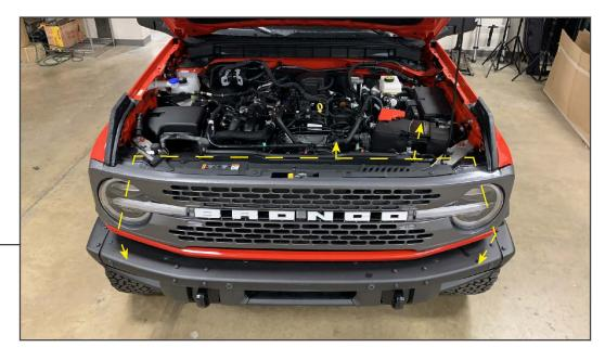
Route the included wiring harness neatly along the engine bay.
