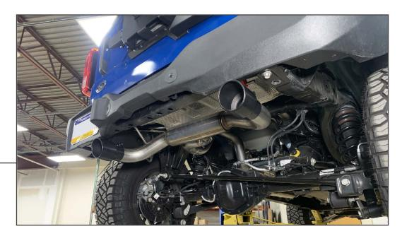
Adjust the exhaust to best fit the vehicle, then tighten all exhaust clamps to 45 ft. lbs.
