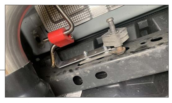
RH Side: Using the included (2) M8 lock nuts, secure the RH side hanger bracket to the pre-existing exhaust hanger studs. Install the (1) rubber hanger once the bracket is secure.
