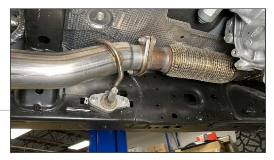
Secure the intermediate pipe to the vehicle front pipe using the original (2) 15mm nuts. Secure the pipe to the vehicle frame using the original hanger and (2) 10mm bolts. Then place (1) 3" exhaust clamp on the end of the pipe.
