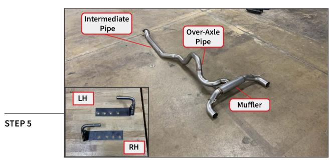
Lay out and identify all exhaust components.
