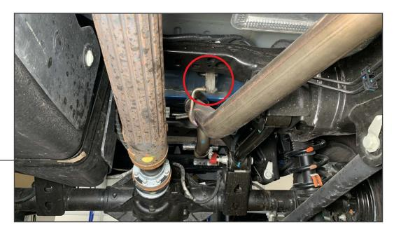
Using spray lubricant and a pry bar, disconnect the (1) rubber hanger supporting the over-axle pipe to the vehicle.
