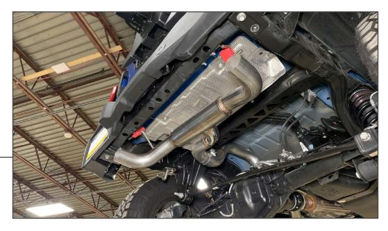
Fit the muffler assembly into the over-axle pipe, and guide each muffler hanger into the rubber hangers.
