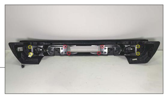
Remove (4) 10mm bolts and (4) 15mm bolts to remove the rear bumper brace to release the fog light harness from the bumper assembly. Remove the proximity sensors, if equipped.
