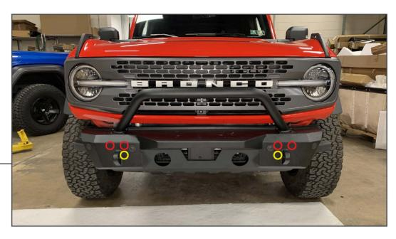
With assistance, lift the bumper to the vehicle frame rails, fitting the studs through the vehicle frame bumper bolt holes. Secure the bumper into place using (2) M12x1.75 x 50mm bolts, (4) M12 nuts, (6) M12 lock washers, and (6) M12 flat washers per side. Adjust the bumper into place, and tighten the mounting hardware evenly until secure.
