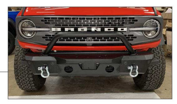
Install the (2) 3/4" D-Rings to the vehicle bumper.
