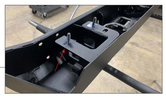
Fit the included (4) stud/nut plates to the inside of the bumper, allowing the stud to fit through the bumper mounting pad. Hold the studs in place using (4) plastic stud holders.
