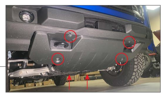
Remove (6) 15mm bolts from the lower splash shield.
