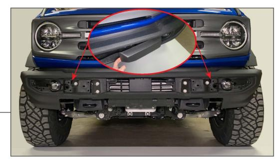
Plastic Front Bumper: Remove the (2) plastic bumper covers using a plastic panel removal tool to reveal the bumper mounting hardware.
