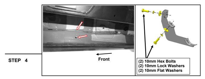
Loosely fit the (1) Passenger Rear step bracket to the vehicle threaded body hole using (2) M10 x 30mm bolt, (2) M10 lock washer, and (2) M10 flat washer. Do not fully tighten to allow for later adjustments.
