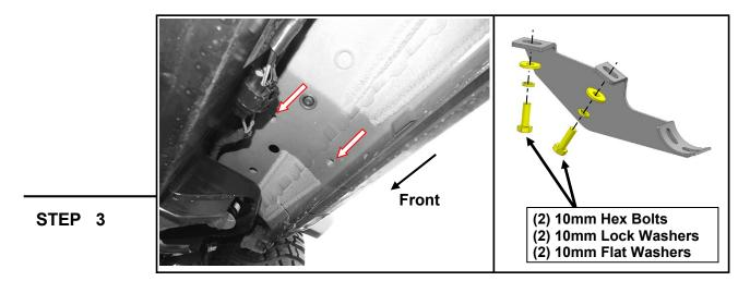
Start installation toward the front of the Passenger/Right side of the vehicle.
