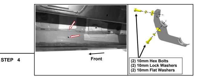
Loosely fit the (1) Passenger Center step bracket to the vehicle threaded body hole using (2) M10 x 30mm bolt, (2) M10 lock washer, and (2) M10 flat washer. Do not fully tighten to allow for later adjustments. Repeat this step for the Passenger Rear step brackets.
