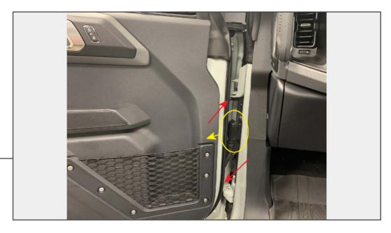
Unplug the vehicle door by pushing the connector cover back, while pulling the wiring harness connector away from the vehicle. Then, remove (1) 13mm bolt from each door hinge. Remove the door from the vehicle and place on a soft surface for storage.
