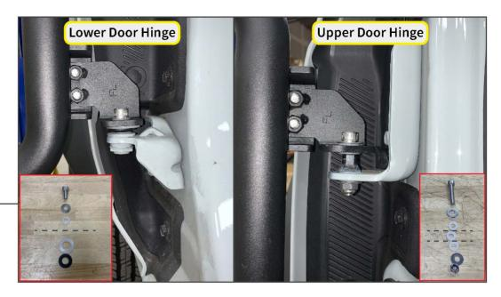
Lift the tubular door onto the vehicle door hinges, ensuring all previously placed washers remain in place.
