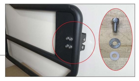
Loosely secure the door latch to the tubular door using (4) M8 x 16mm bolts, (4) M8 flat washers, and (4) M8 nylon washers. Ensure the nylon washers are in-between the flat washer and the vehicle door.
