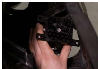
4. Install your new SS3 pod using the factory hardware. The tabs and holes on the bracket should align with the mounting points of the factory fog light housing. Re-use the factory hardware, tightening securely.
