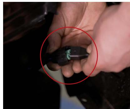
5. Use the included wire adapters to connect the pod to the vehicle wiring harness. Test function. If the light does not turn on, try flipping the connector 180°.
