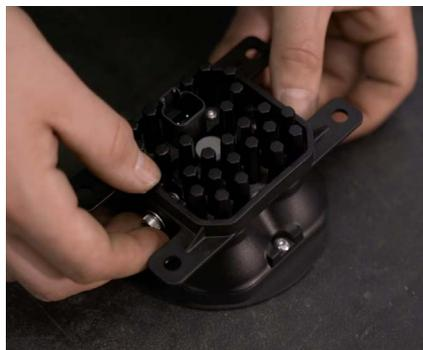
1. Install the supplied nuts into the pod housing with the nylon facing inward. Attach the bracket to the pod using the supplied screws and washers. Make sure the bracket is in the correct orientation. See diagrams above. Ensure that the screws are tightened such that the pod retains its position, but can pivot with force for aiming.
