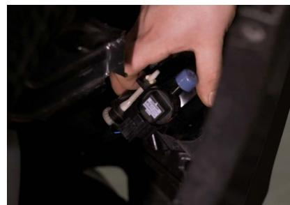
3. Disconnect the fog light connector from the vehicle wiring harness. Remove the factory fog light housing. The factory hardware will be reused.
