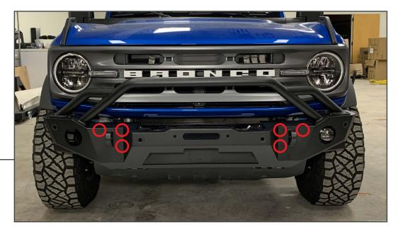
Place the (2) M12 bumper mounting nut plates behind the vehicle frame rails. With assistance, lift the bumper to the vehicle frame rails. Secure the bumper into place using (3) M12x1.75 x 50mm bolts, (3) M12 lock washers, and (3) M12 flat washers per side. Adjust the bumper into place, and tighten the mounting hardware evenly until secure.
