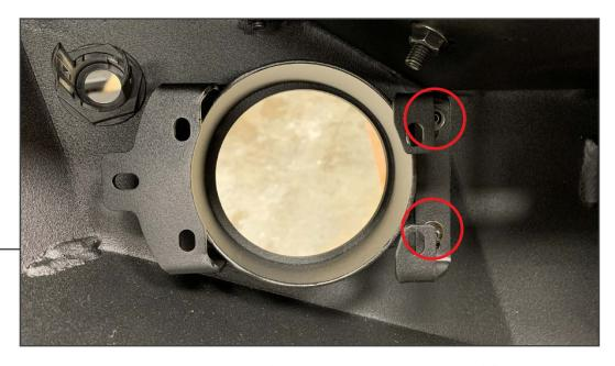
Install (1) fog light mounting bracket to the bumper fog light mounting pad using (2) M4x0.7 x 15mm Allen bolts, (2) M4 lock washers, and (2) M4 flat washers.
