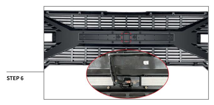
**Forward Facing Camera:** Using cutters/rotary tool, carefully cut the square section located at the center of the grille. The necessary cutout section will appear similar to the cutout in the OEM grille. Cut minor sections at a time to ensure a proper fit.
