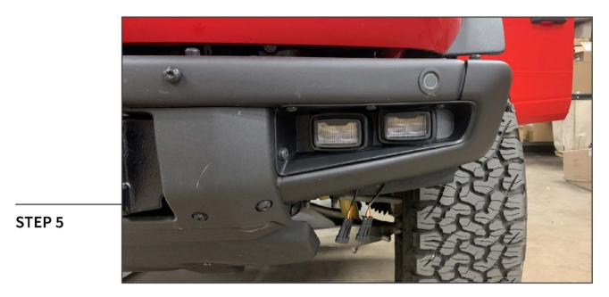
Adjust each light assembly using the knobs attached to each light housing. Re-install the wheel well liner using the original hardware.
