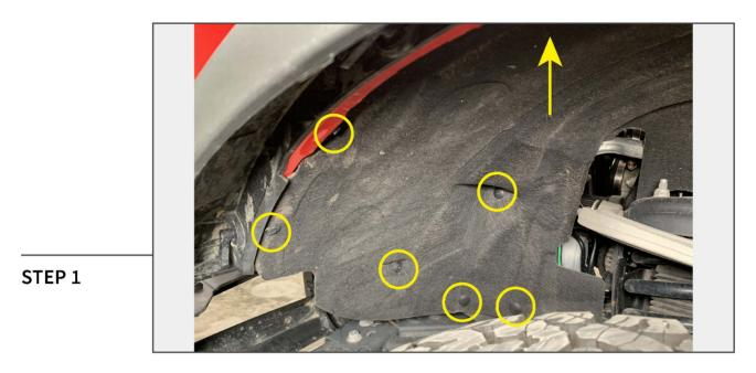
In the vehicle wheel well, remove the front fasteners from the wheel liner.
