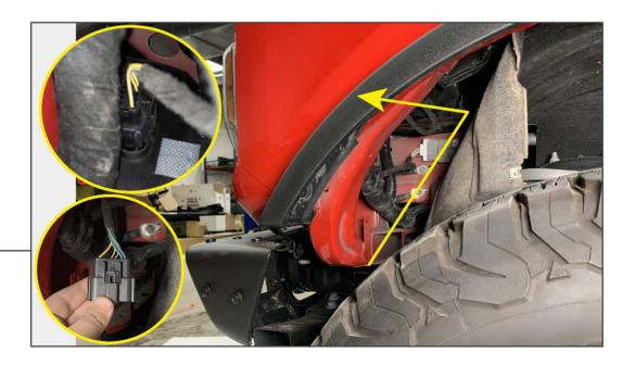
Reach upwards behind the vehicle headlight and unplug the headlight wiring harness.
