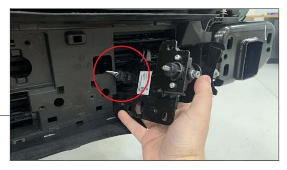
Unplug the ACC module from the shutter assembly wiring harness.
