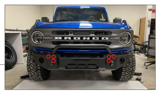
Place the (2) bumper mounting nut plates behind the vehicle frame rails. With assistance, install the bumper to the vehicle frame rails using (6) M12 x 65mm bolts, (6) M12 flat washers, and (6) M12 lock washers. Do not fully tighten to allow for adjustment later.
