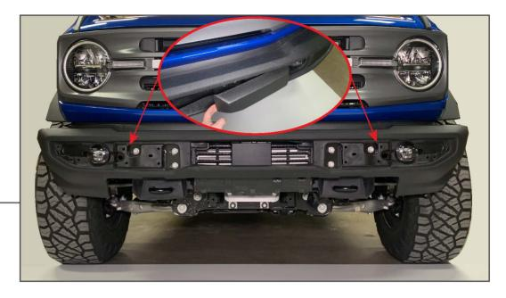
Remove the (2) plastic bumper covers using a plastic panel removal tool to reveal the bumper mounting hardware.
