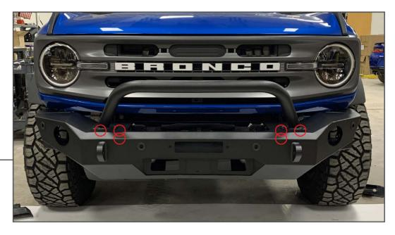
Fit the (2) M12 nut plates behind the vehicle frame rail. Then, lift the bumper to the vehicle frame rails. Loosely secure the bumper into place using (6) M12x1.75 x 50mm bolts, (6) M12 lock washers, and (6) M12 flat washers.
