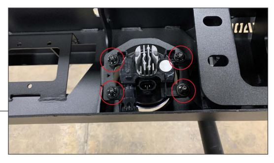
Secure the OEM fog lights to the vehicle bumper using (4) M6x1.00 x 20mm Hex bolts, (4) M6 flat washers, and (4) M6 flange nuts. Tighten all hardware evenly until secure.
