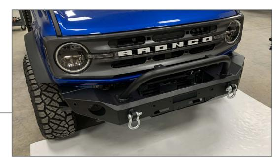
Install (2) 3/4" D-Rings to the vehicle mounting points. Neatly route the bumper wiring harness along the bumper/vehicle.
