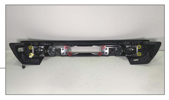
Remove (4) 10mm bolts and (4) 15mm bolts to remove the rear bumper brace to release the fog light harness from the bumper assembly.
