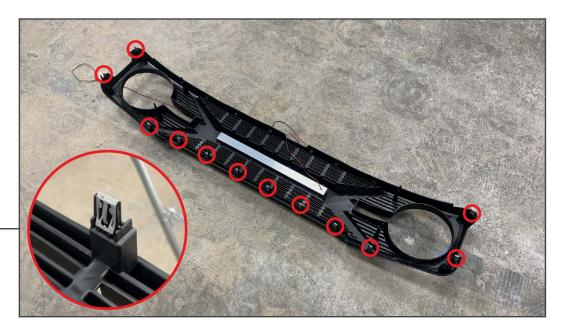
Fit the (12) new metal retaining clips to the grille clip posts.
