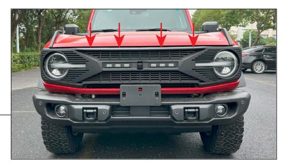
Secure the top of the grille to the radiator support using the original (4) 10mm bolts. Tighten until secure.
