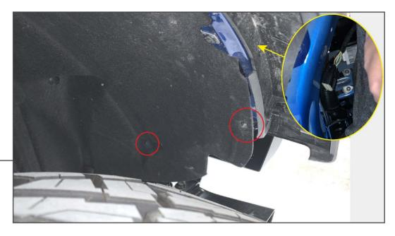
Remove (2) Phillips head plastic push clips from the front of the wheel well liner on each side of the vehicle. With the clips removed, reach up and unplug each headlight electrical connector.
