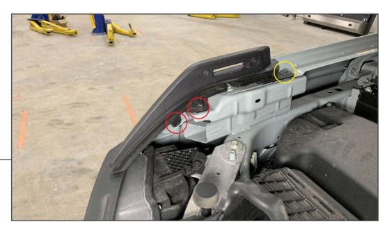
Open the vehicle hood. Remove (2) 10mm nuts and (1) 10mm bolt from the hood tie down assembly. Lift and remove the assembly from the vehicle.
