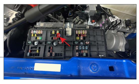
Open the vehicle fuse box, and locate the indicated fuse. Remove the fuse and plug in the DRL fuse tap harness. Neatly route the harness and close the fuse box.
