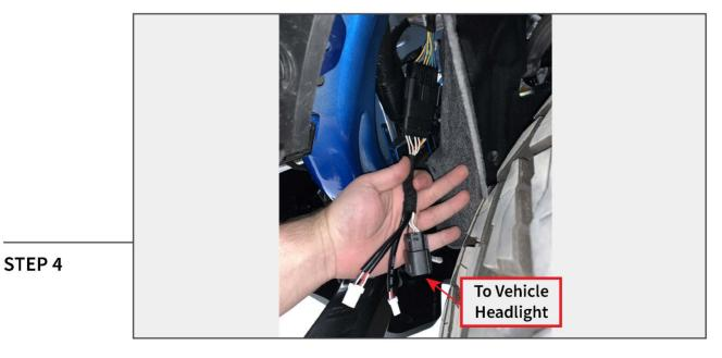
Plug the "T" harness into the vehicle headlight wiring harness connector, then plug the "T" harness into the vehicle headlight.
