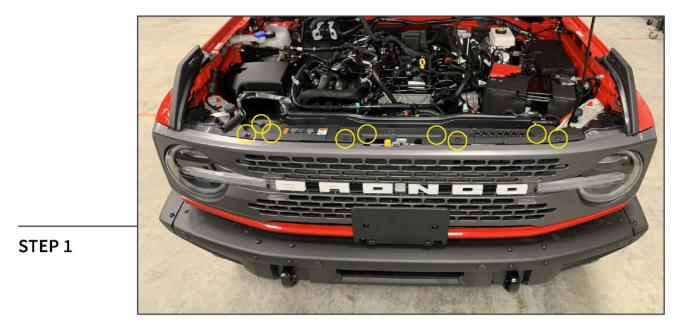
Open the vehicle hood. Locate the front radiator trim panel. Remove (9) plastic push clips from the radiator trim panel using a panel removal tool.
