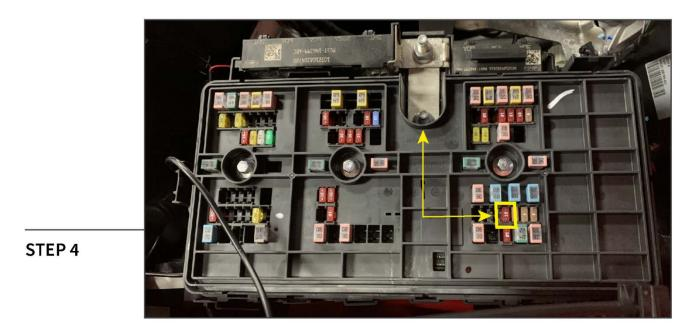
Remove the fuse box lid. Locate and remove the indicated fuse from the fuse box. Insert the (1) fuse tap into the fuse slot. Connect the ground terminal on the wiring harness to the vehicle battery ground/suitable vehicle ground. Re-install the fuse box lid. The lights will power on with the ignition on.
