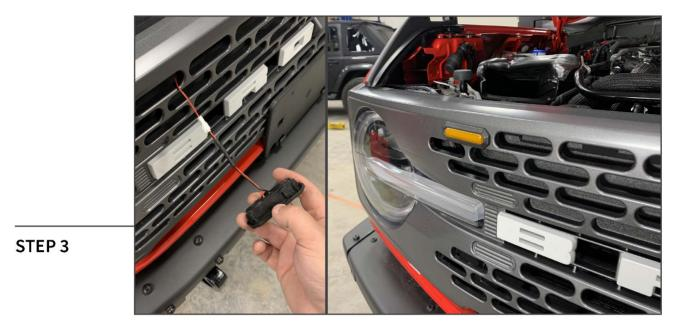
Identify the (3) LED lights based on the label located on the back side of the light assembly (left [Driver's Side], middle, right [Passenger's Side]). Plug in the corresponding light to the harness, and press the LED light into the grille assembly until an audible click can be heard to confirm light engagement in the grille. Repeat this step for the remaining LED lights.
