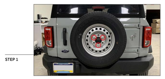
Remove the vehicle spare tire using a lug wrench, and set the spare tire aside.
