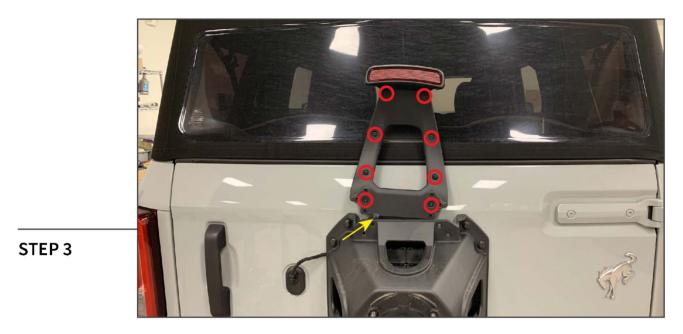
Slightly lift the tail light enclosure over the tire carrier, and disconnect the wiring harness retainer from the enclosure using a pry tool. Then, remove (8) T-25 Torx screws from the tail light enclosure. Gently use a pry tool to separate the tail light enclosure assembly.
