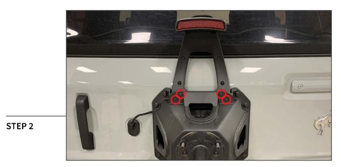
Remove (4) T-30 Torx screws to disconnect the third brake light enclosure from the tire carrier.
