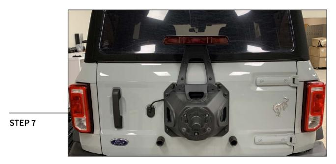
Plug the new third brake light into the vehicle wiring harness, and neatly route the wiring harness into place. Re-assemble the third brake light enclosure using the original hardware. Ensure the wiring harness is not interfering with assembly.
