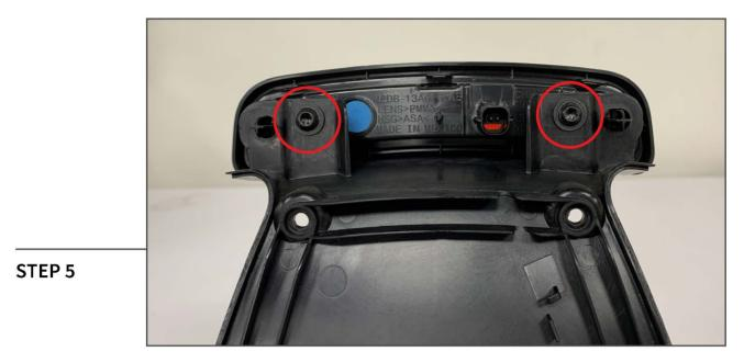
Remove (2) T-25 Torx screws from the vehicle third brake light. Remove the original third brake light from the enclosure.
