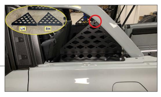
Identify the (2) window mounting brackets. Each bracket is side specific. Secure each window bracket to the vehicle roll bar using (1) T-45 Torx bolt and (1) M8 flat washer. Do not fully tighten to allow for bracket adjustments later.
