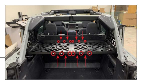
Secure the (2) horizontal braces to the trays using (20) M6 bolts and (20) M6 nuts.
