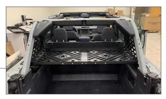
With all components in place, tighten all hardware evenly until secure.
