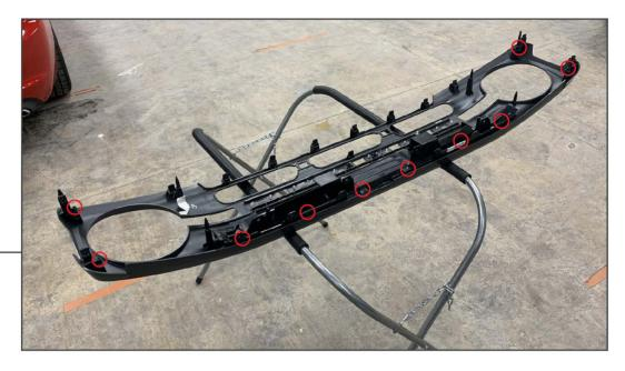
Along the outer edge of the grille, remove (10) T-25 Torx screws, and remove the plastic panels from the grille.
