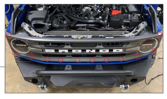
Firmly pull the grille away from the vehicle to dislodge the (12) metal retaining clips. Once the grille is removed, place the grille on a soft surface for disassembly.
