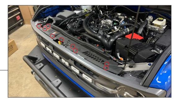
Open the vehicle hood. Remove (9) plastic push clips from the upper plastic trim. Remove the trim panel from the vehicle.
