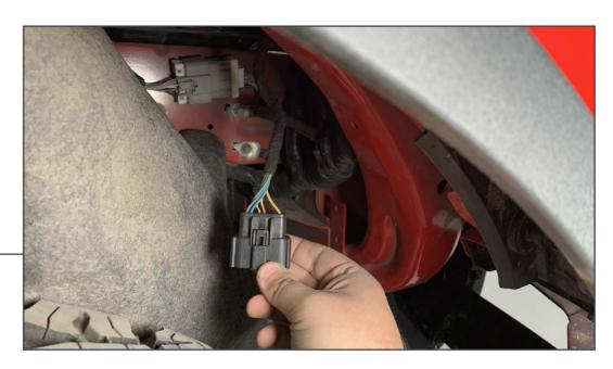
LED Light Wiring: Wire the grille lights to the vehicle RH side headlight harness using the following diagram. Splice into the harness using the included scotchlok connectors. The lights will power on with the parking lamps. Fender liner may need to be partially removed for better wiring access.
