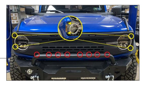
Align the grille to the vehicle, and align the dowel pins attached to the grille to the vehicle dowel retainers. Route the wiring towards the RH side headlight assembly, away from any hot/moving components. Once aligned, fit the grille into the vehicle metal clip retainers across the bottom of the radiator support and the side fenders.
