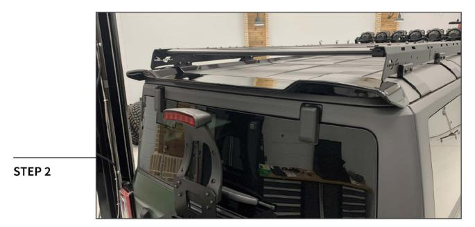
Test fit the spoiler to the vehicle prior to removing the red tape backing to familiarize fitment. Once familiar, peel the red tape backing and firmly press the spoiler to the vehicle hard top.
