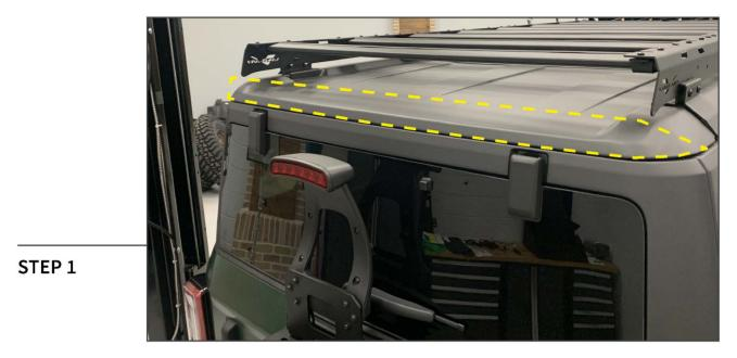
Clean the vehicle hard top first with the (2) alcohol prep pads and allow to fully dry. Then, clean the same area using the (2) adhesion promoter pads and allow to fully dry.
